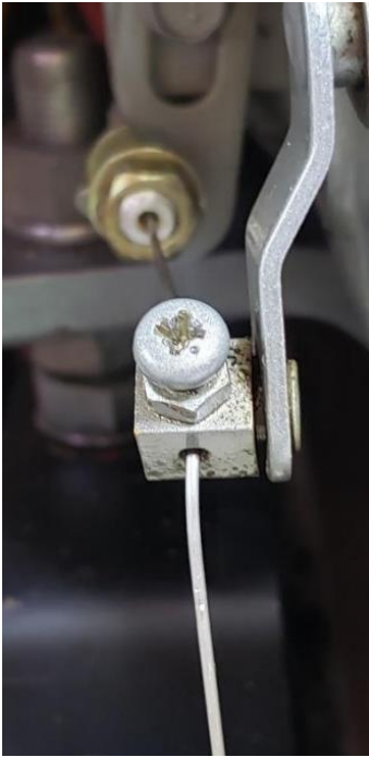
Figure 3: Screw head starting to strip.
